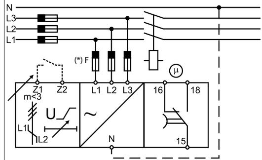
Connect the 3-phase power supply and the neutral (if present) taking care of the sequence. Connect the relay output according to the ratings.
